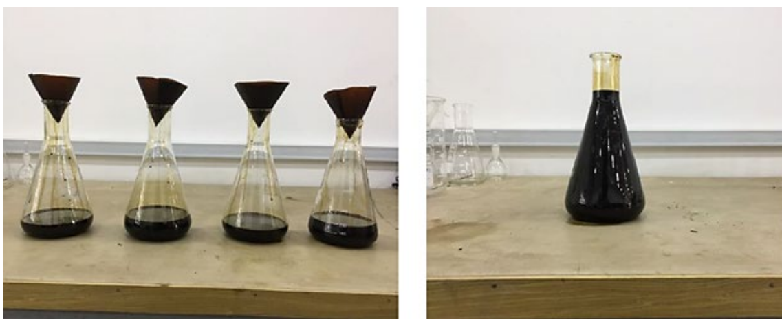
Fig. (7): Crude oil recovery from sorbent materials (PSBC).
