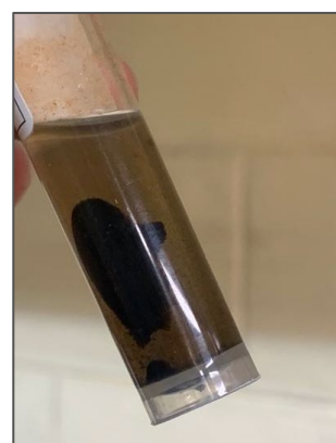
Fig. (7): The change in colour represents the first indicator for nanoparticle formation in the reaction vessel
