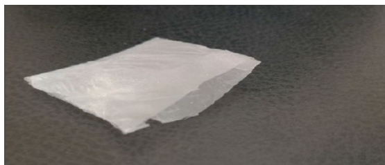
Fig. (7): The Shape of Plastic Bags After Manufacturing Them by Hot-gluing Their Edges and Preparing Them for Food Preservation Testing.
