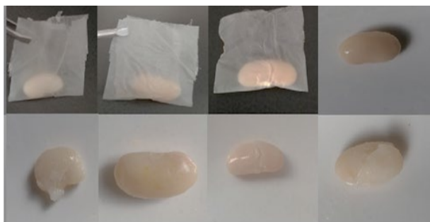
Fig. (8): The Effect of Preserving Beans by Using Prepared Bags with Biofilms: (1) P3HB/M, 2) P3HB/G, (3)P3HB/C, and (4) not Using them as A control Element After 72 hrs.
